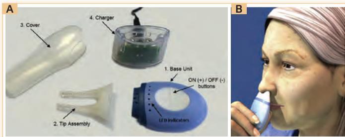
**Figure 5.** Intranasal tear neurostimulation. (A and B) A handheld device features 2 prongs that are inserted into the nostrils to deliver electrical stimulation to the trigeminal nerve to promote tear secretion.<sup>16</sup> (C) Stimulated and unstimulated mean Schirmer scores.<sup>15</sup> Differences were significant at  $P < .0001$  at all timepoints ( $n = 40$ ). (D) Corneal staining scores in the same study as in Figure 5C.<sup>15</sup>
