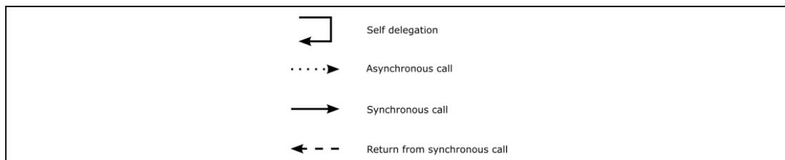
The diagrams uses slightly modified UML symbols. The asynchronous call is not depicted as suggested in UML. Some objects do have more than one dashed line. It symbolizes more than one thread.
