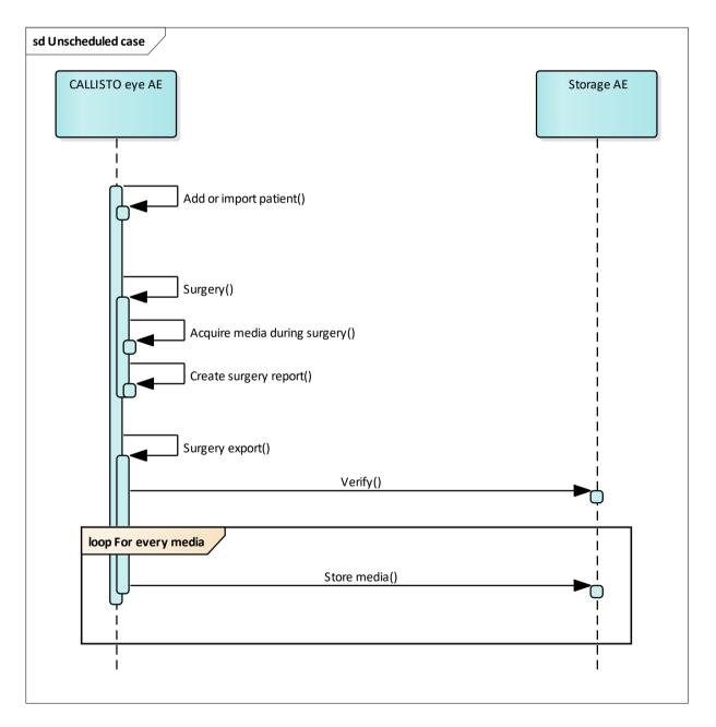
Main activities are initiated by an operator. The sequence diagram shows different phases. An operator triggers the activities in the planning phase (Import IOLMaster or FCW Scheduling Object via USB, FCW Scheduling Object via WLAN, CSV Import or add patient manually) and the export phase (Surgery export).
