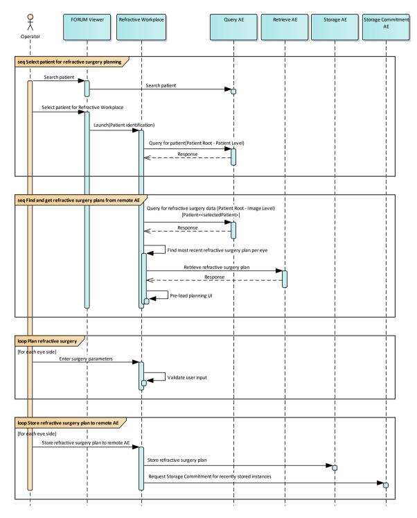
Figure 4-5 Standard workflow
