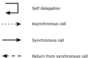
The diagrams use slightly modified UML symbols. The asynchronous call is not depicted as suggested in UML. Some objects do have more than one dashed line. It symbolizes more than one thread.
