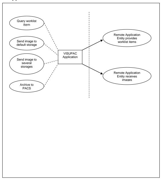
The VISUPAC Application, runs the User Interface for the operator. Here, the VISUPAC Application is located on a Capture Station or on a Viewing Station. From there an operator can perform the Real-World Activities "Query worklist item", "Send image to default storage" and "Send image to several storages".
