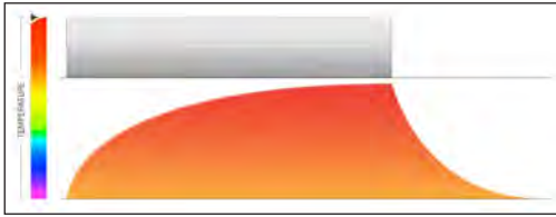
Figure 3: Schematic of the temperature rise associated with a continuous wave laser application. The gray bar represents the duration of the laser pulse and the orange-red represents the rise and fall of the temperature of the treated tissues.
