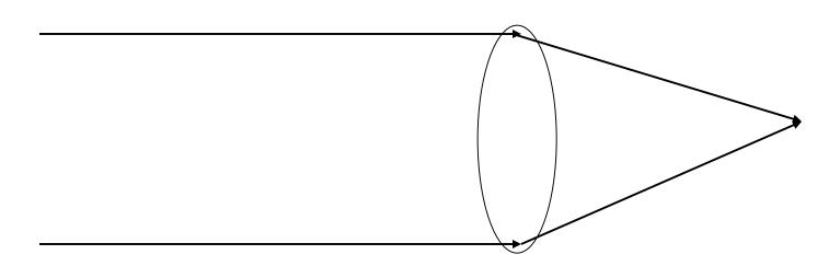
In this example, a plus lens causes previously parallel rays to converge to a point
