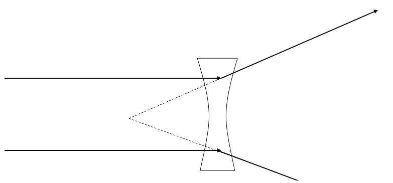
In this example, a minus lens causes previously parallel rays to diverge from a point
