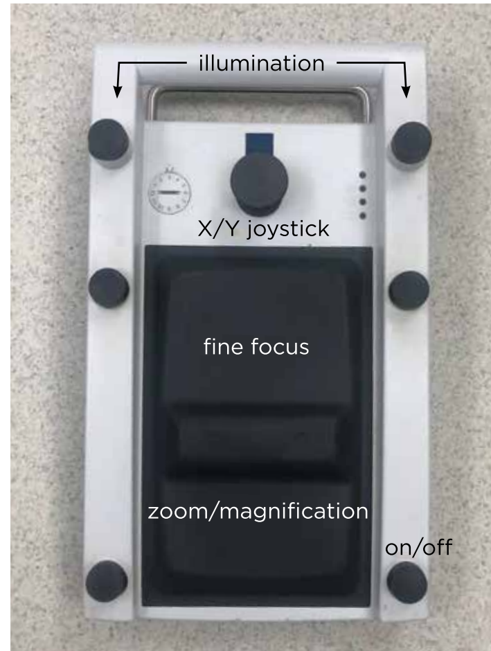
Operating microscope foot pedal. Functionalities can differ slightly based upon type of microscope used.
