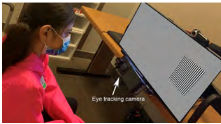
Figure 1: A child with cortical visual impairment (CVI) performs eye tracking in the Chang laboratory at the Saban Research Institute at Children's Hospital Los Angeles. The eye tracking camera (arrow) uses infrared light to calculate the direction of eye gaze with high precision while the child watches visual stimuli on a computer monitor.
