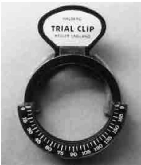
FIGURE 12–16. Halberg clip-on lens holder.
