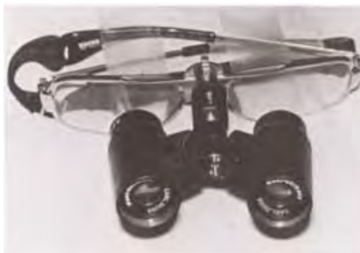
Figure 17 Zeiss telescopic loupes mounted on a sturdy spectacle frame with an elastic head strap
